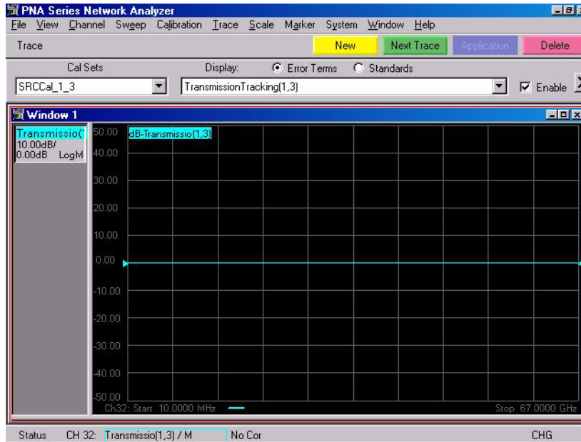
Figure 53 SRCCal Transmission Tracking(1,3) Normalized
