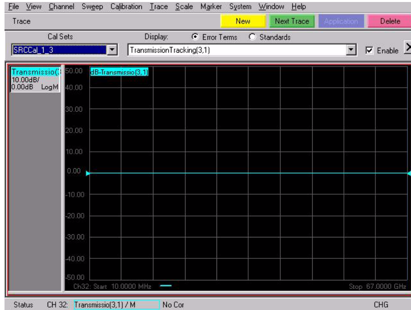
Figure 57 SRCCal Transmission Tracking(3,1) Normalized
